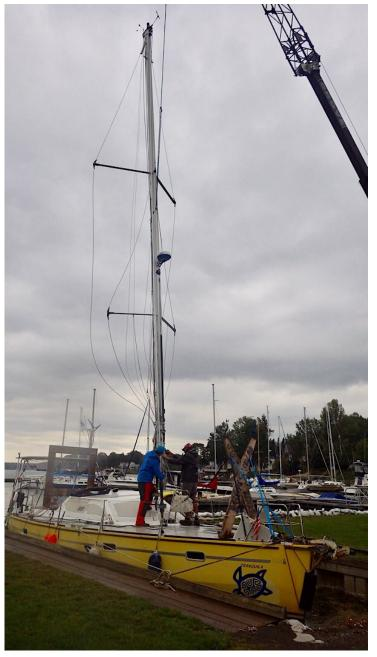
We now need to tighten all the stays & get the boom back up. We managed to get it down using the halyards and the boom topping lift (looked that one up!) so hopefully we'll be able to get it back up the same way.
